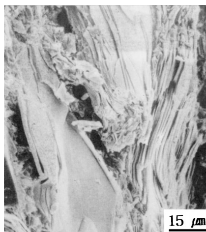
Figure 2 Fractograph of the compounds hot pressed at 420 °C.
